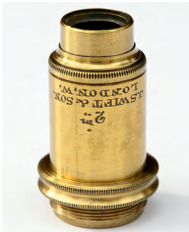
Figure 4. An antique two-inch achromatic microscope objective manufactured by James Swift & Son of London in 1858 which was used to create the image in Figure 3.
