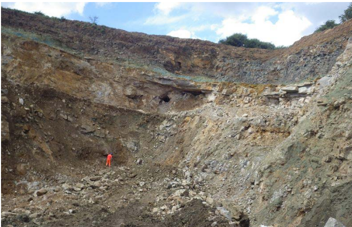
Fig. 1. Basalt lava and ash over dipping dolomitic limestone and old mineworkings. Steve Critchley for scale.
