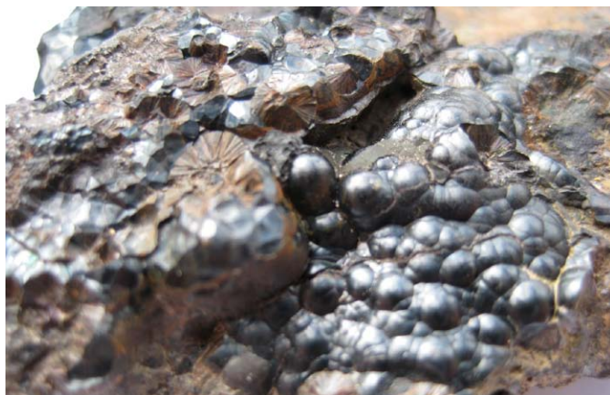
Figure 5. Goethite showing internal radiating structure. The sample is 8 x 3 cm.
