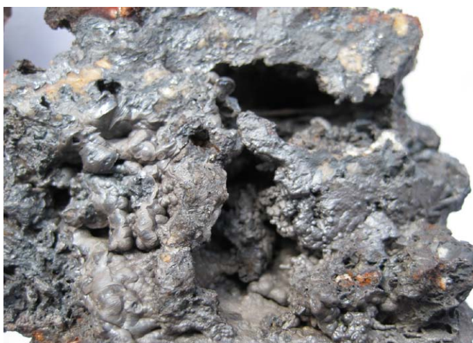
Figure 6. A sample of dark brown-black cellular ore. A complex mix of iron (± manganese) oxides. The sample is 7 x 5 cm.
