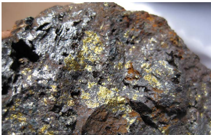
Figure 2. Sample of partially altered primary chalcopyrite and chalcocite (silvery-grey-top left in photo).The sample is 8 x 3.5 cm.
